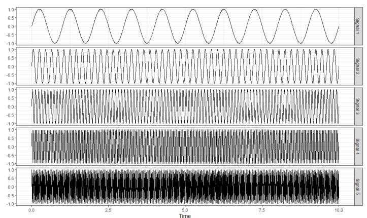
The five signals are combined together to generate a mixed frequency signal, which we can use with PSD estimation to show signal decomposition. Further, we add simulated noise/error by adding a gaussian random sample (SD = 1) to our combined signal. We also use a band-pass (3 Hz - 30 Hz) finite impulse response (FIR) filter to show how we can target a specific range of frequencies for analysis (Helwig, 2018).
