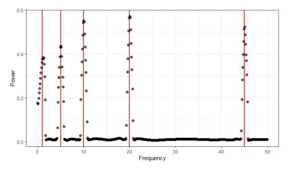
Next, we apply a 3-30 Hz band-pass FIR filter, to showcase the effect of isolating specific frequencies of interest. After applying the bandpass filter, we see that the power distribution in all frequencies outside the region of interest are near zero, and that we can still estimate the 3 frequencies present in the signal which were within the filter region.
